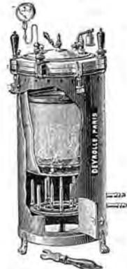
Fig. 331. Autoclave Chamberland.
