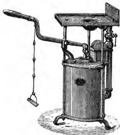
Fig. 344. — Forge double-vent.
